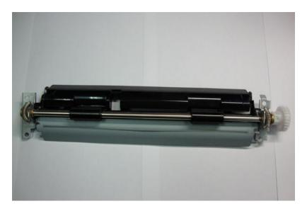
3. Remove the shield from the feed roller assembly, reinstall the feed roller in the printer.
